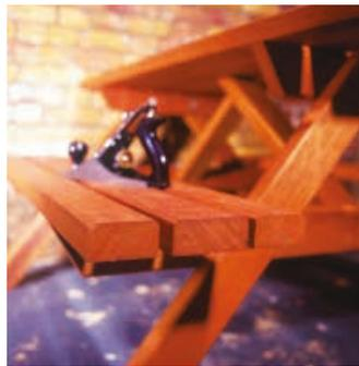
**2 Cutting the table and benches.** Cut 12 lengths of timber the length of your bench, using the plane to chamfer them lengthways, removing the sharp edges, until they are smooth to the touch.
