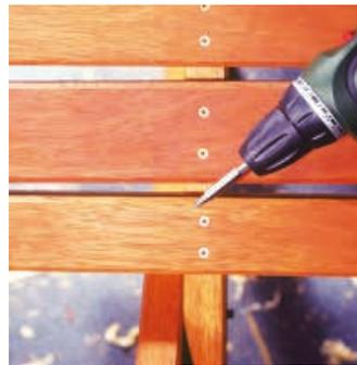
**3 Fixing the table and benches.** Countersink, glue & screw six of these lengths, equally spaced, to the tops of the two A frames, to form the table top. Do the same for the next three for each bench, as shown.
