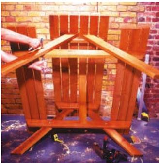
**1 Making the frame.** Cut two lengths of timber to your desired table top width, cutting each end at a 45 degree angle. Do the same for two lengths of timber to the overall width for the table and bench together. Cut four lengths of timber with 45 degree ends long enough to form the legs. Bolt these pieces together as shown to form an A frame (pre-drill and countersink the coach bolts).
